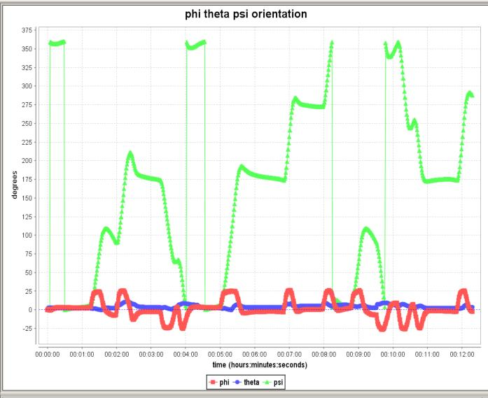
Rotational angles (phi theta psi) time-series plot. Rotational angles (phi theta psi) measured about world-coordinate axes (+X+Y+Z) respectively. Units are degrees/second versus mission time. Positive values rotate according to the right-hand rule.
