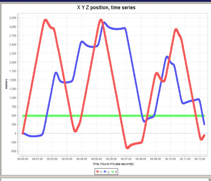
X Y Z telemetry time-series plot. Robot coordinate system: world coordinates for vehicle position. +X (North), +Y (East) and +Z (down) data in meters versus mission time.
