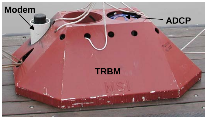
Figure 10: An acoustic modem and acoustic Doppler current profiler (ADCP) were housed in a trawl-resistant bottom mount (TRBM) during AOSN-II.
