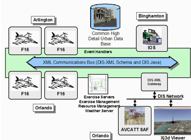
**Figure 8. Link Four F16 Ownship Demonstration Configuration**
