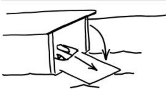
Figure 7. Storyboard sketch of landing craft exiting the well deck of an amphibious ship.
