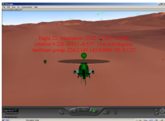
Figure 1. Multiple helicopters, tanks and humanoid avatars move and interact within the NPS Capture-the-Flag research application, a synthetic battlespace on Fort Irwin terrain (45x55km 2 ), rendered here using Netscape Navigator, CosmoPlayer VRML 3D plug-in, and DIS-Java-VRML networking.
